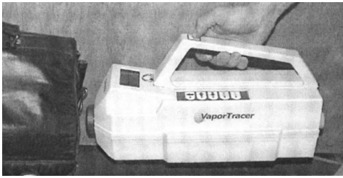
Fig. 22 The GE Infrastructure Security VaporTracer sniffing a briefcase
