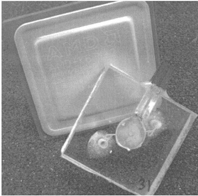
Fig. 12 A 10 mm pump chamber with 300- \mu\text{m} -wide optimized Tesla valves from Table 2. The pump body is acrylic, and a PZT-5A actuator is bonded to a 270- \mu\text{m} -thick polycarbonate membrane. The electronic computer chip indicates its intended application.
